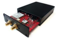
The TM-R9B3 / R9A10 is a mid-range product line member of KCS' advanced TraceME track and trace modules. The TM-R9B3 is targeted for remotely tracing and controlling vehicles and other powered equipment.
